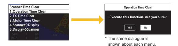
Save the following scanner time data stored in the scanner into the display unit.
