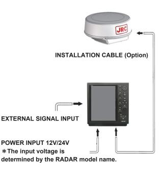
Connect the arrows in the diagram. (For inputting external signal, optional NMEA cable is required. Refer to chapter 1.2.6.)
