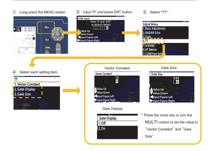
Vector Constant: Vector shows the movement of the target. When Vector Constant is large, vector is stable, but the response is slow. When Vector Constant is small, vector is unstable, but the response is quick.
