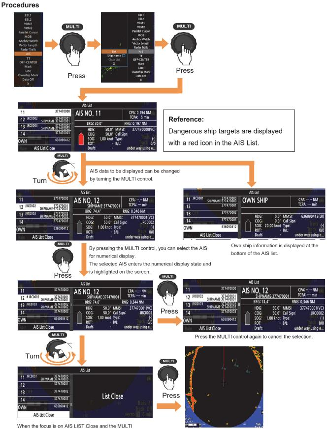
control is pressed, the display of the AIS list ends. Even if you exit the AIS List, the AIS information in the numerical display state will be displayed continuously.
