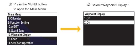
When the function is turned on, the waypoint mark is displayed on the radar screen as red circle. It is connected Onwship and a Waypoint with a straight red line.
