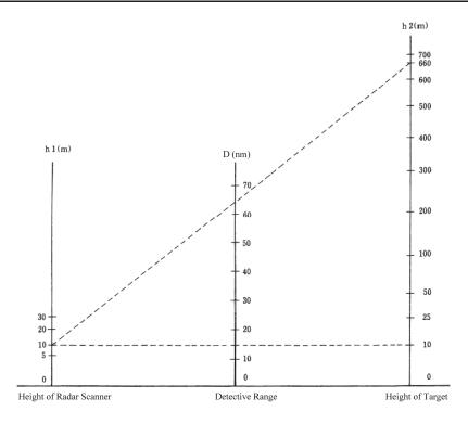
When the height of own ship's scanner is 10 m for instance,
