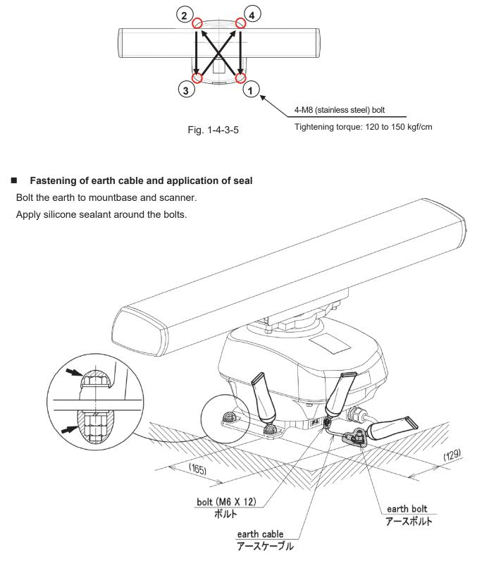
To uniformly press the packing, gradually tighten diagonally in the following order.
