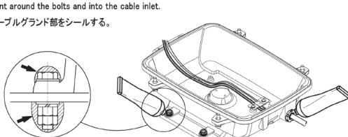
Bolt the earth cable to mountbase and scanner. Apply silicone sealant around the bolts.
