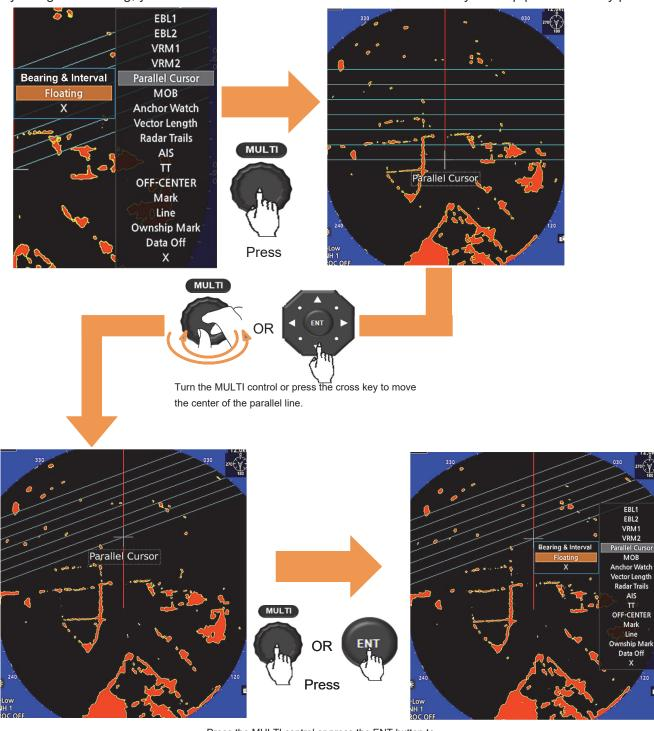
Press the MULTI control or press the ENT button to set the center point at the moved position.
