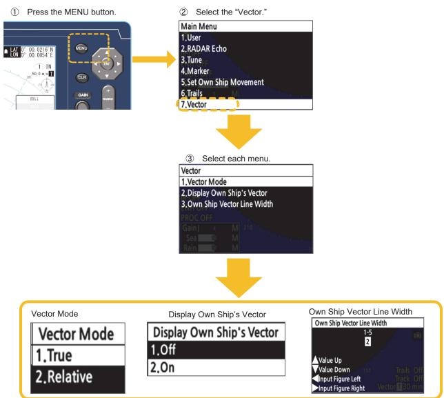
To display the vector, you need to input the direction and speed signal.
