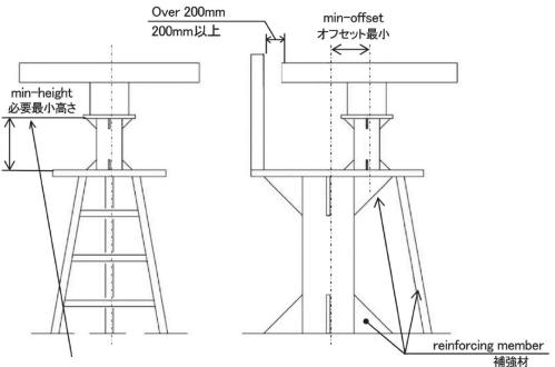
Set up a scaffolding for maintenance if the minimum height shown above is 1 m or more.
