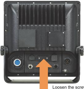
Loosen the screws (2 pcs.), and remove the cover. Connect DVI cable.
