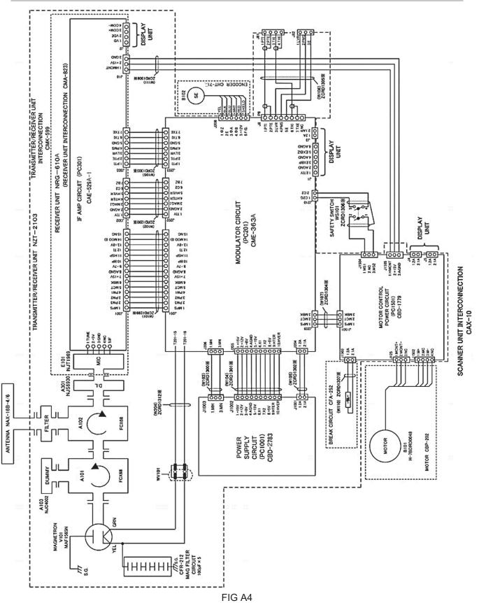
**NCD-2364 DISPLAY UNIT INTER CONNECTION DIAGRAM**
