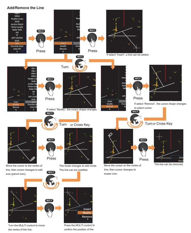
The Line function memorizes the position using latitude and longitude. GPS position information signal must be input. Therefore, this function cannot be used unless GPS is input. If change the color or type of the line, see "5.31 LINE SETTING."
