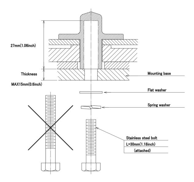
% FIX THE BOLTS BY USING A STANDARD WRENCH (LENGTH 135mm TORQUE 2058[N·cm])
