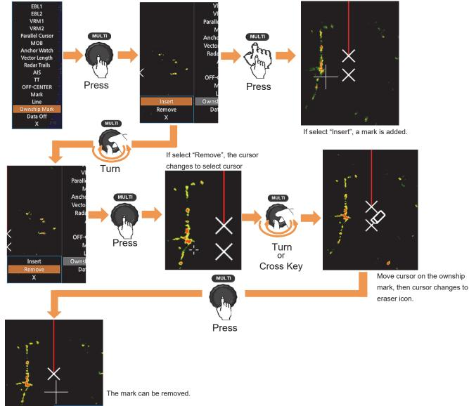
The Ownship Mark function memorizes the position using latitude and longitude. GPS position information signal must be input. Therefore, this function cannot be used unless GPS is input. If change the size, color or type of the mark, see "5.30 OWNSHIP MARK SETTING."
