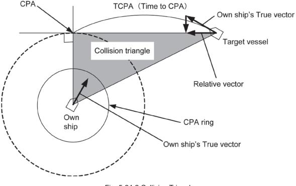
Fig. 5-24-2 Collision Triangle
