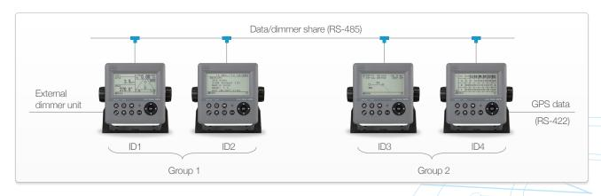
In this sample, the display with ID4 receives data (RS-422) from sensor or optional junction box and outputs vessel position data (RS-485) to all connected display. Dimmer share has been separated in two groups, whereas group 1 can be operated by external dimmer and group 2 is linked pressing the button on the display.
