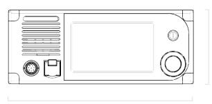
240 mm \*Flushmount cut out (9.44 in) 215 mm x 89 mm
