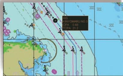
the vessels, and bearing, range, speed, length, heading and much more AIS target specifics from other ships are received and displayed. The AIS symbols are continuously displayed on-screen without the influence of the radar characteristics. The AIS targets are never shielded by ground, rain or cloud reflections, nor are they eliminated by adjustments of anti-sea or anti-rain clutter.
