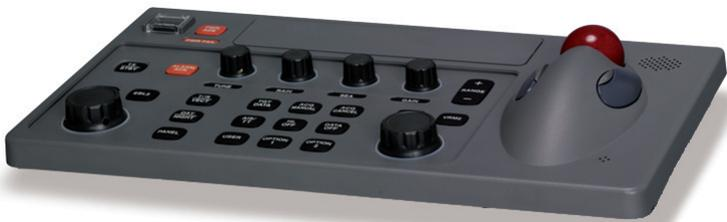
The responsive feel keys allow logical and precise operation and also integrate function keys for one-touch access to VIDEO, RAIN, SEA and GAIN. This makes it seamless to navigate through all commonly used tasks.
