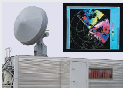
A Doppler radar system capable of detailed, three-dimensional measurements of rain cloud structures
