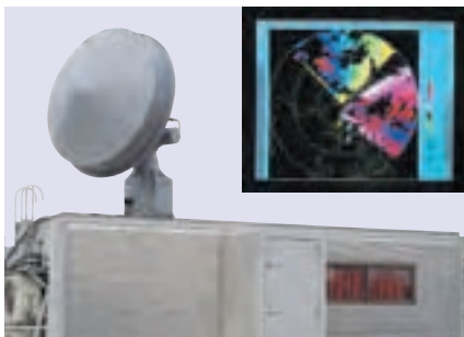
A Doppler radar system capable of detailed, three-dimensional measurements of rain cloud structures
