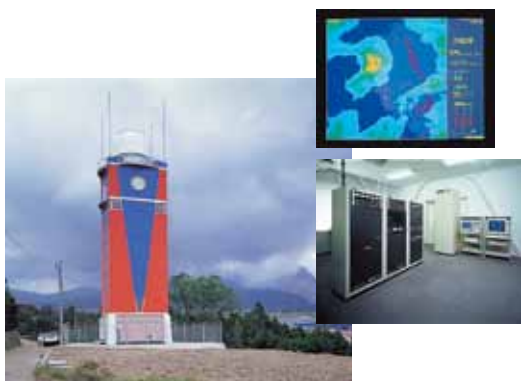
A small radar system capable of detailed measurements, even for local rain showers
