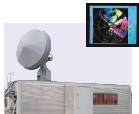
A Doppler radar system capable of detailed, three-dimensional measurements of rain cloud structures
