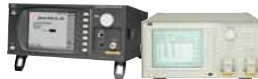
Application tester (NJZ-4000) for HSDPA and W-CDMA and multi-path fading simulator (NJZ-5000)
