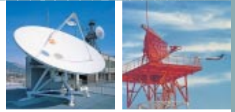
Disaster prevention radio communication system (satellite network system) Airport surveillance radar system
