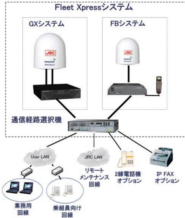
図2 Fleet Xpressシステム構成 Fig.2 Fleet Xpress system Configuration
