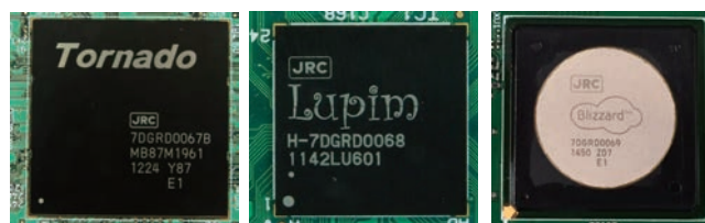
図2 自社開発レーダー用LSI Fig.2 Radar LSIs Developed by JRC
