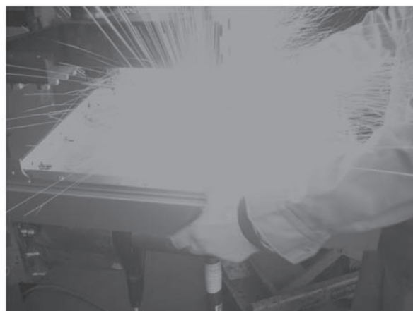
図5 溶接時の爆飛 Fig.5 Explosion Welding
