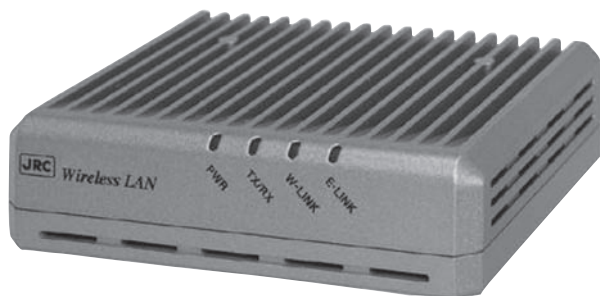
図3 4.9GHz帯無線LAN装置 (据置型) Fig.3 4.9GHz WLAN (fixed installation type)
