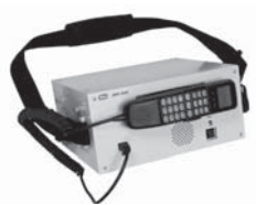
図4-3 半固定局無線機 Fig.4-3 Portable station radio equipment
